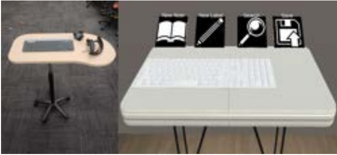
Fig. 2. Left: Keyboard stand with wireless keyboard, HTC Vive Tracker, and example space for a controller. The keyboard is on a wheeled table which allows the participant to move the keyboard around the space as needed during their analysis. Right: Virtual representation of the keyboard. Attached to the keyboard are four menu options. These options from left to right are New Note , New Label , Search , and Save . These menu options are attached to the table and will move with the table as it is moved around the space.
