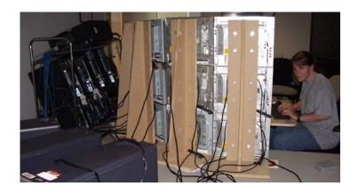
Figure 2: Cluster of twelve computers running the 24 panel, 31.5 megapixel display.
