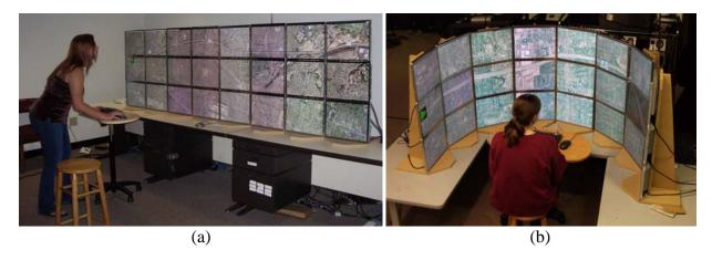
Figure 4: 24 panel, 31.5 megapixel display in the flat (a) and curved (b) configurations in experiment 1
