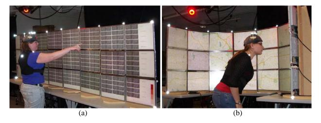
Figure 11: The 24-panel, 31.5 megapixel display in the flat (a) and curved (b) configurations in experiment 2. Participants stood, and their physical navigation was tracked by the Vicon system overhead.
