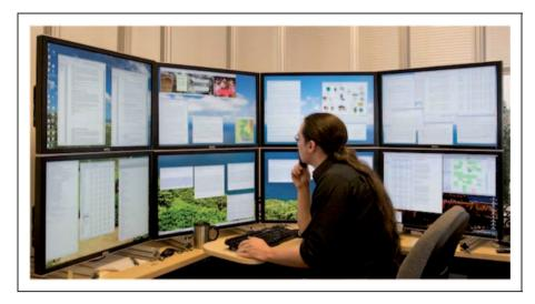
Figure 2. An alternative form factor (curved) large, high-resolution display functioning as an everyday workstation.
