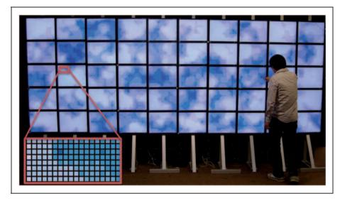
Figure 1. A 50-display tiled large, high-resolution display.
