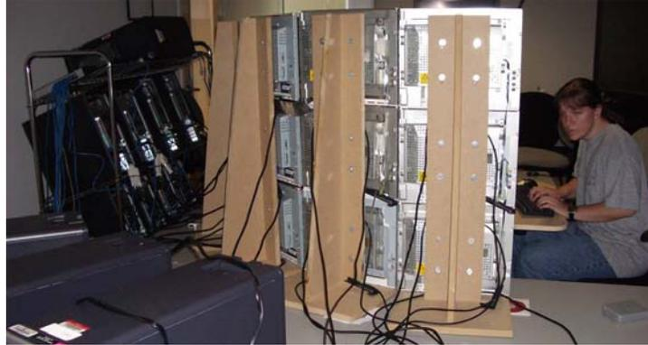
**Figure 2: Cluster of twelve computers running the 24 panel, 31.5 megapixel display.**
