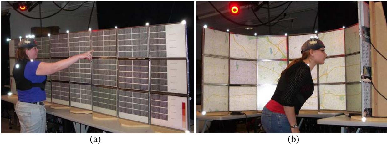
**Figure 11: The 24-panel, 31.5 megapixel display in the flat (a) and curved (b) configurations in experiment 2. Participants stood, and their physical navigation was tracked by the Vicon system overhead.**
