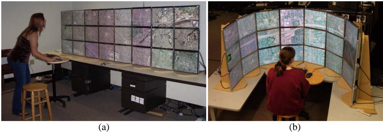
**Figure 4: 24 panel, 31.5 megapixel display in the flat (a) and curved (b) configurations in experiment 1**
