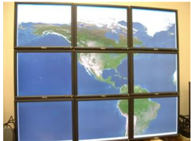
Figure 1: The nine-monitor tiled configuration. The total resolution is 3840x3072 (11,796,480 pixels).
