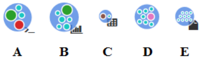
Figure 3: Five different types of output badges: (A) text output, (B) chart, (C) table, (D) no output, (E) file output. The size difference of the nodes corresponds to the frequency with which the cell components are used in the overall notebook.
