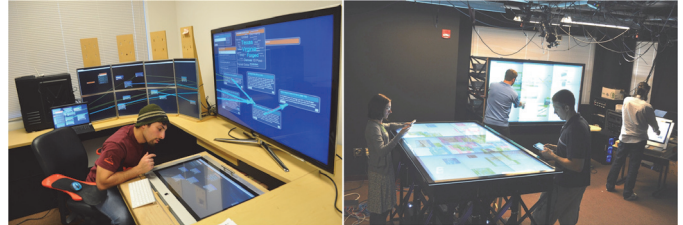
Fig. 1. Display Ecologies for Visual Analysis: Personal Display Ecology (Left) [1] and Collaborative Display Ecology (Right) [3].
