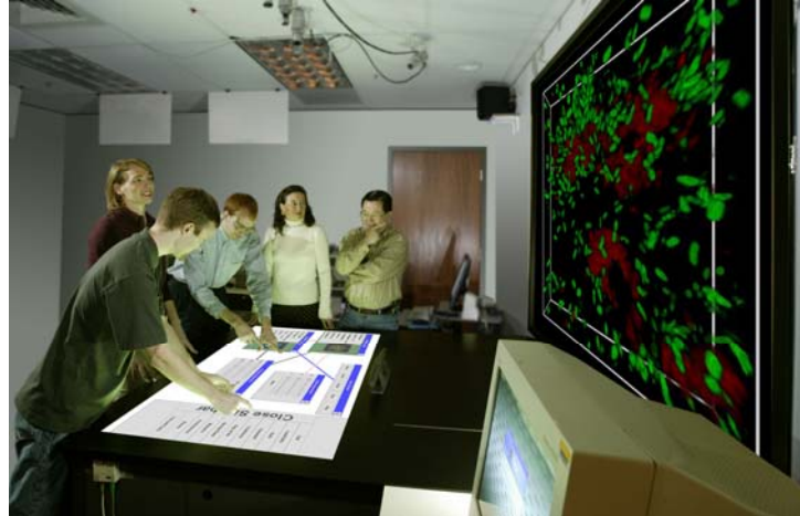
HI-Space users interacting with 3D geometry data generated from 48 confocal microscope image slices at 512x512 resolution.
