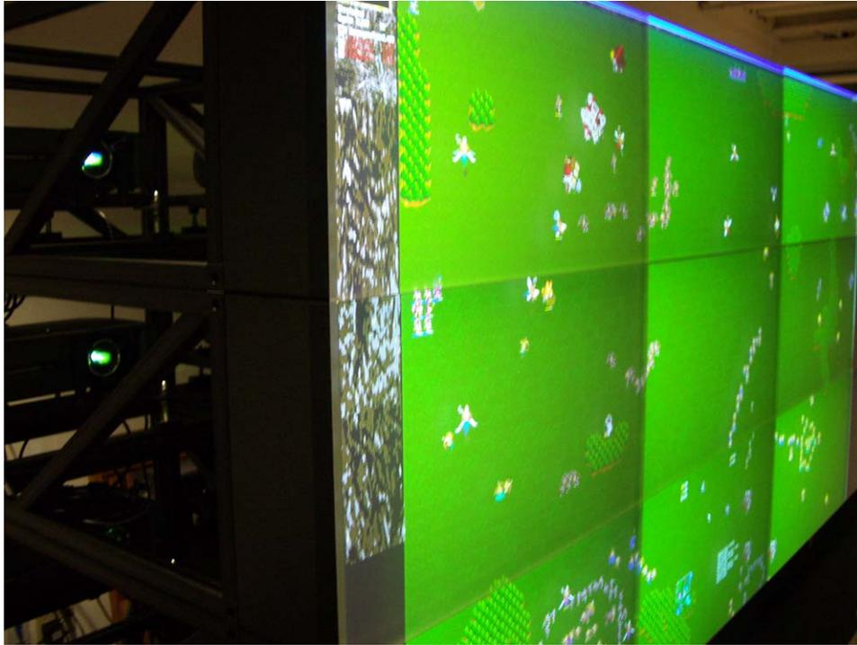
*Figure 12. Wargus running on a rear-projection display at a resolution of 3840x2160.*
