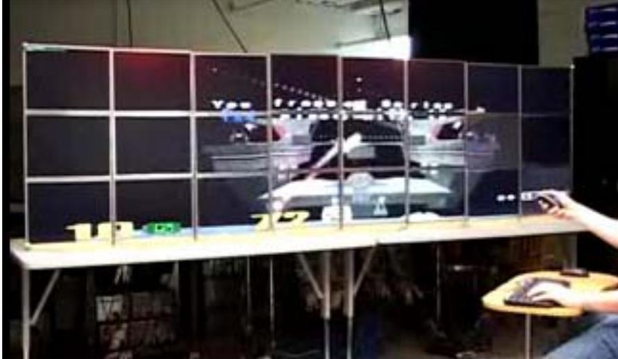
*Figure 21: Quake 3 being played on a flat 24-monitor display wall with a gyro mouse.*
