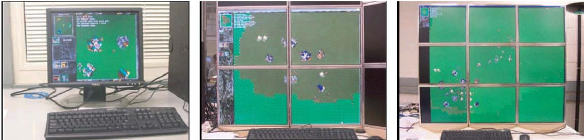
*Figure 2. One-monitor (640x480), four-monitor (1600x1200), and nine-monitor configuration (2400x1800).*
