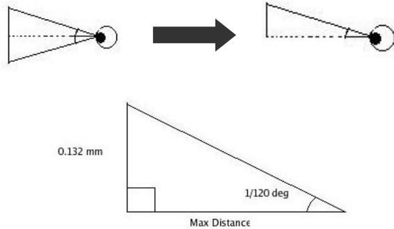
Figure 3: Right Triangle for Calculating the Maximum Resolvable Distance from a Pixel
