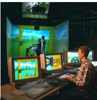
Figure C10: Deere & Company's VR testing facility for virtual prototyping vehicle designs and testing their effectiveness (Photo courtesy Deere & Company, Moline, Illinois [27]).
